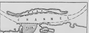
The drawing below shows the way in which the channels at Oranjestad harbor will appear after the dredging operations have been completed. The filled area will be used as the concrete break extension to the pier. With two channels deep enough for large ships it will no longer be necessary for them to turn around inside the harbor to leave by the same entrance they entered.
